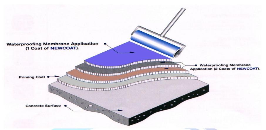
A new age innovative waterproofing system – No breaking of existing Brickbat Coba
